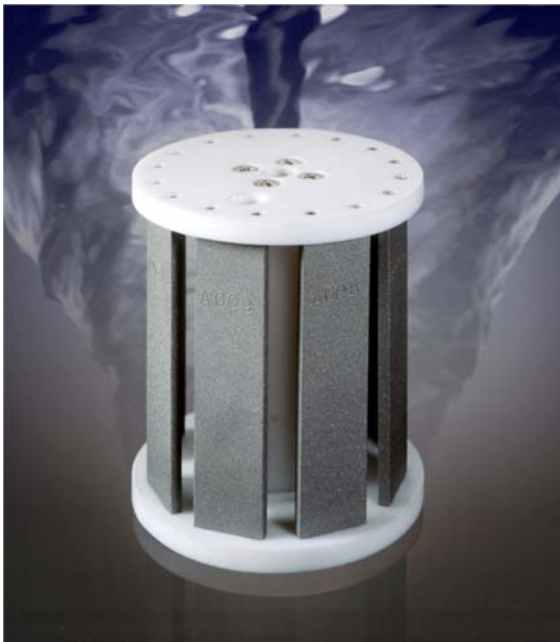
FIG. 2 Photo of Rotating Cage Containing Coupons
